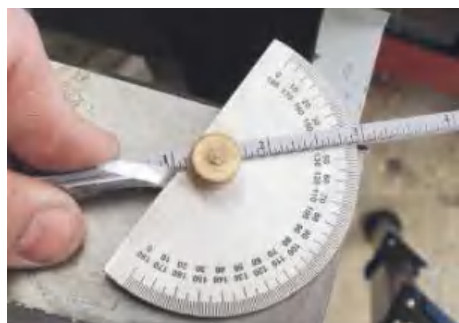
▲ Pic.5 A good working angle on the spindle gouge is around 40°. Going to 35° would be better for shaping and going to 45° would be better for hollowing
